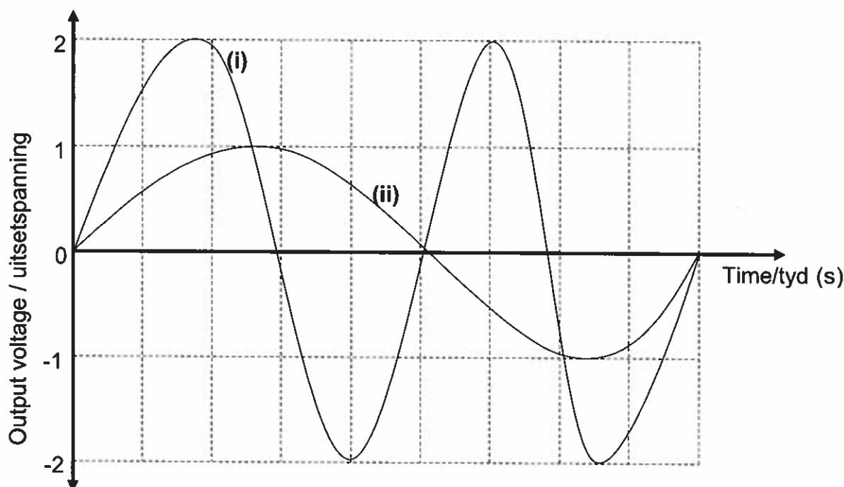
Both the frequency and magnitude of the output voltage are proportional to the speed of rotation. Hence, at half the rate of rotation, ✓ the frequency and magnitude would be also be halved✓ (as shown in the graph (ii))
