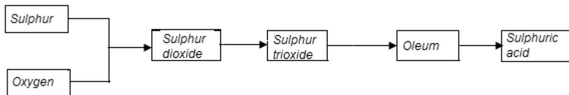
Flow diagram of Contact process
