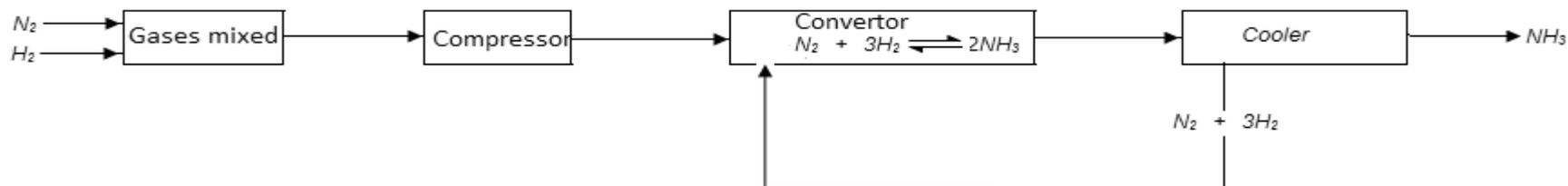
From the cooler, ammonia is collected as a liquid. Unreacted nitrogen and hydrogen are sent back to the converter.
